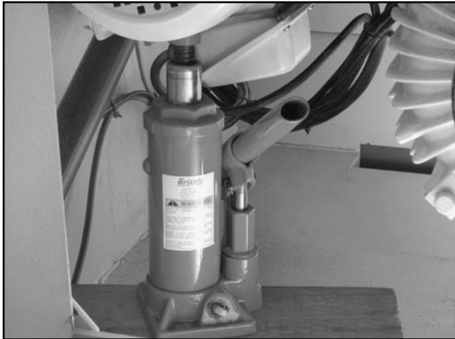
Figure 91. Jacking up scoring motor with a bottle jack to remove the belt.
